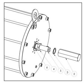
The setting of the closed valve position is performed by adjusting the screw which is inserted into the end flange of the pneumatic cylinder as follows:
