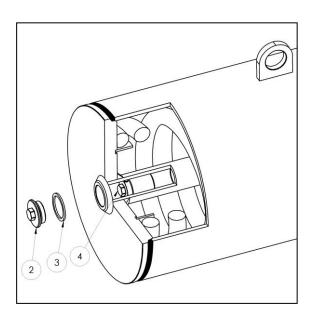
The setting of the open valve position is performed by adjusting the screw which is screwed into the spring pack:
