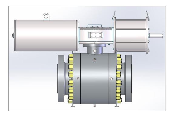
Assembling by interposing an adapter and a coupling joint.
