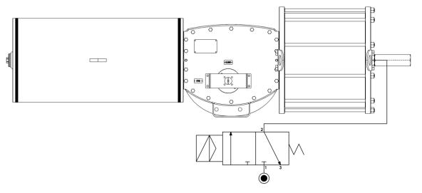
Attention: the customer must take precautions to prevent the actuator chamber unmanned does not aspire from the outside air not filtered, moisture, water or other substances harmful for the actuator.
